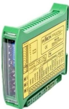
Amplifier WG09 is dedicated to work with linear displacement sensor (LVDT). Amplifier feeds sensor and convert its output signal to analog amplifier's signal 0÷10V or 4÷20 mA and also to digit signal in standard RS485 Modbus RTU. The device has calibration keys which enable calibration with any sensor to any measuring range. Additionally amplifier enables internal and external temperature measurement (fe. temp. of LVDT). The device has an rail mounted enclosure DIN 35mm standard.
